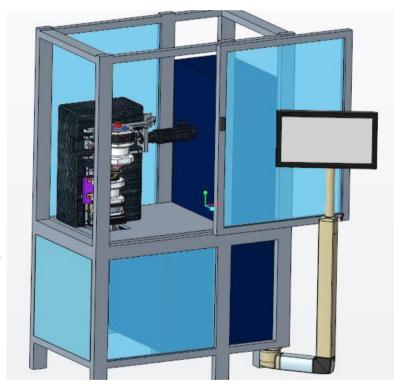
Spindles are aligned in vertical direction to ensure a proper clamping. Due to their large cross section, the spindles are positioned on opposite sides. As benefit we can handle small distances between axis, as well as inspection of internal gears.
